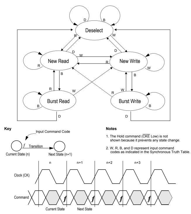
Current State and Next State Definition for Pipelined and Flow through Read/Write Control State Diagram
