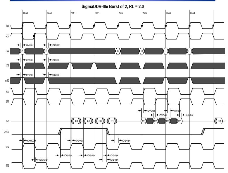
Note: The DQ = High-Z states depicted in this diagram apply when DQ input termination is disabled (MZT = 00). See page 13 for the DQ state timing diagram that applies when DQ input termination is enabled (MZT = 01 or 10).
